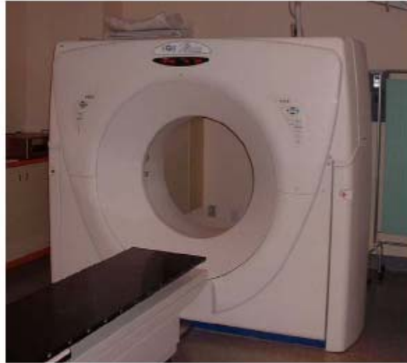
Figure: A dedicated radiotherapy CT simulator. Note the flat table top and the large bore (85 cm diameter). The machine was manufactured by Marconi, now Philips.
